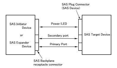
Figure 1.2 Example of SAS system configuration (Dual port internal backplane environment)
